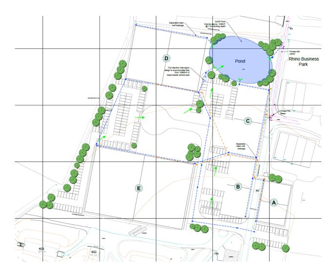
It is intended that storm water is held within a Sustainable Urban Drainage Systems SUDS. On this site this would work by water being stored within the pond with a volume of at least 1445m2.
